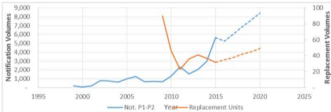
Figure 47: High Priority Notifications vs. Replacement – DSS Transformers
