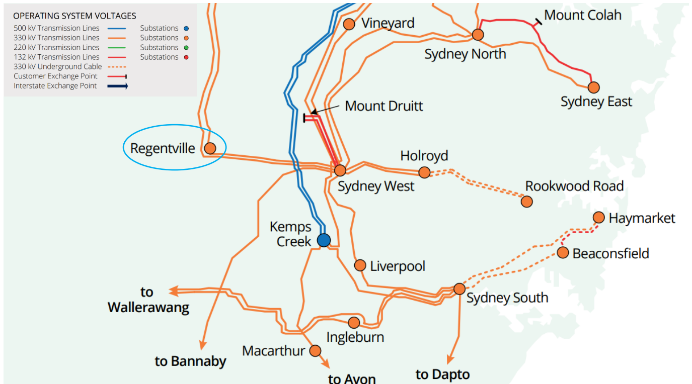
Figure 1: Central NSW transmission network
