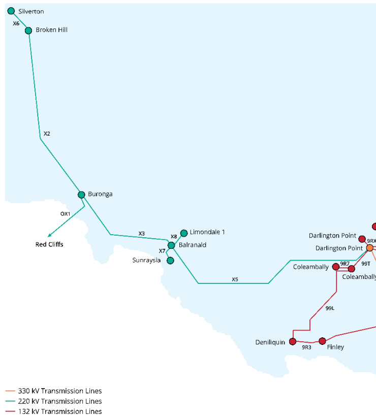
Figure 1: Transmission network in far west NSW
