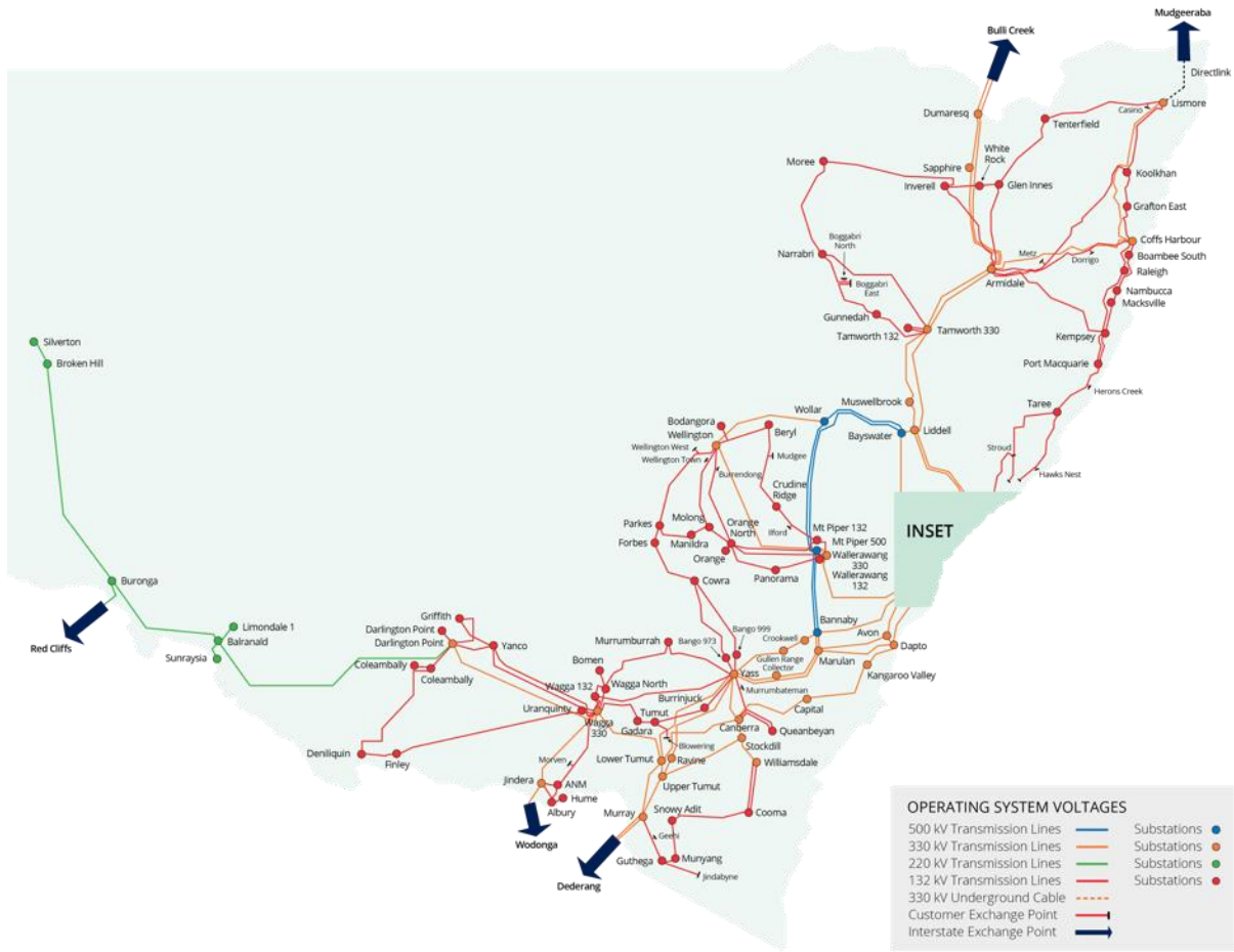
Figure 4-1: Transgrid's electricity network map
