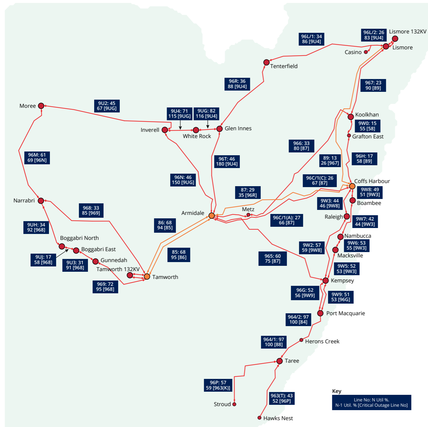
Figure A4.6: TransGrid N and N-1 line utilisations – North Coast and North West 132 kV System
