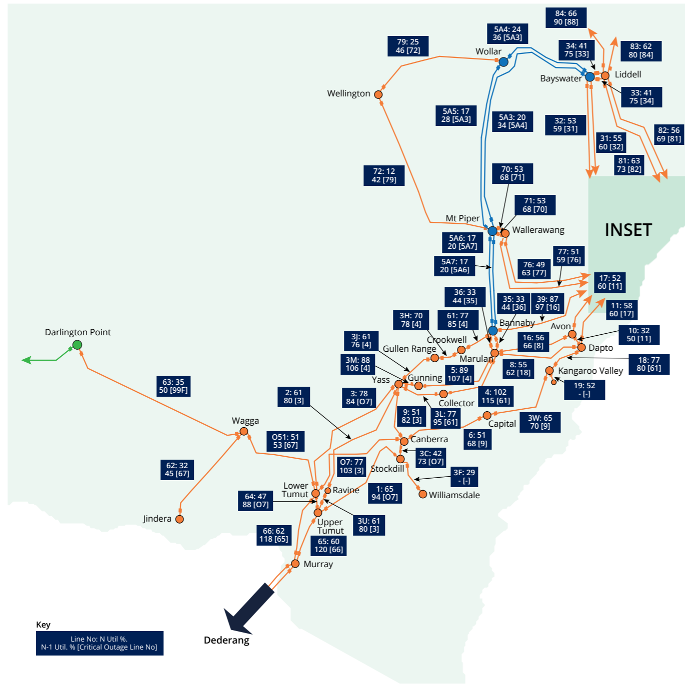
Figure A4.4: TransGrid N and N-1 line utilisations – South and South East
