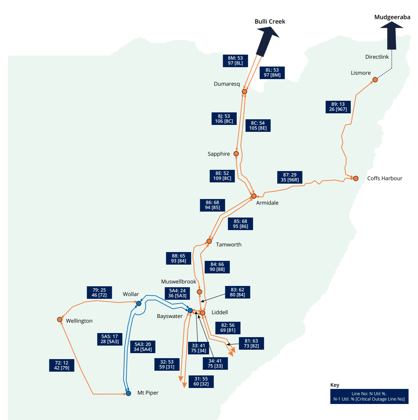
Figure A4.3: TransGrid N and N-1 line utilisations – North East NSW and Northern NSW
