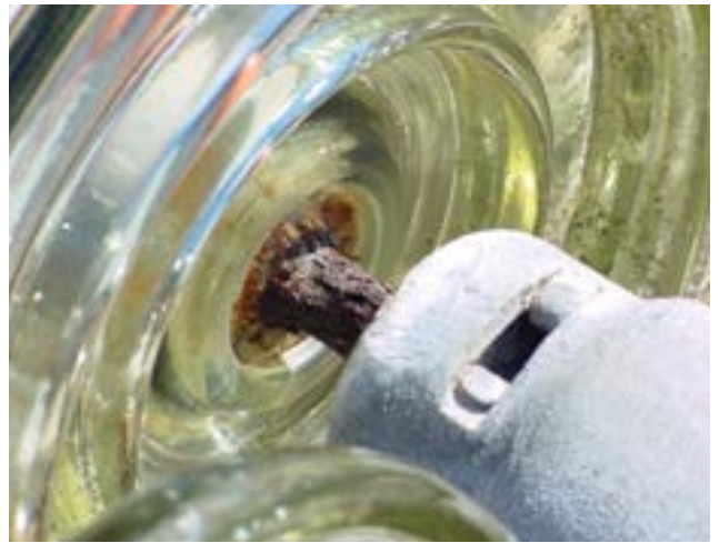
A worn insulator
