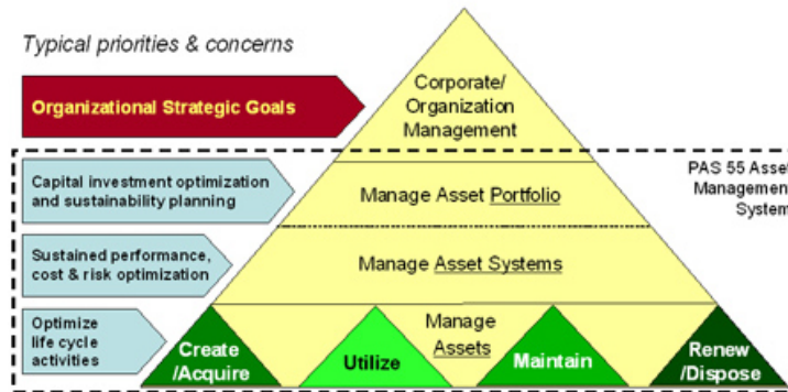
Figure 2 Overview of the PAS 55 asset management standard
