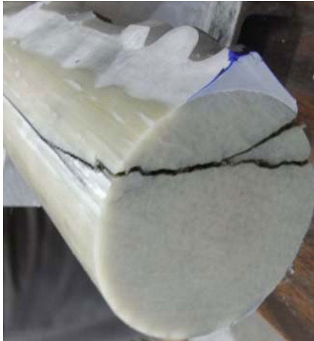
Figure 7 Cracking of fibreglass rod of insulator on TL446T232 (2013 failure) 2
