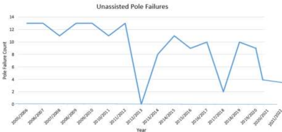
Figure 9 TasNetworks owned unassisted pole failures trend
