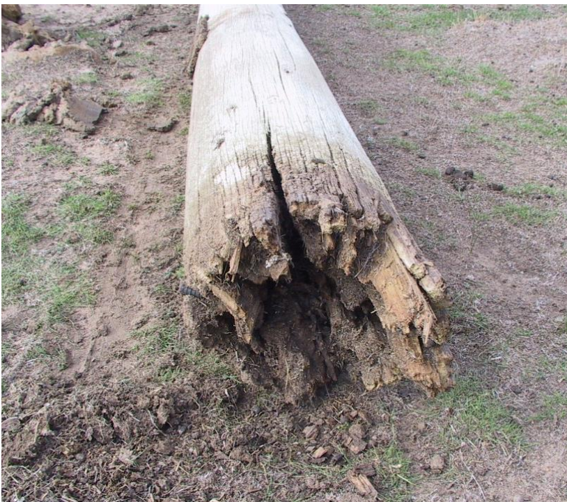
Figure 15: Wood Pole that has Failed in Service
