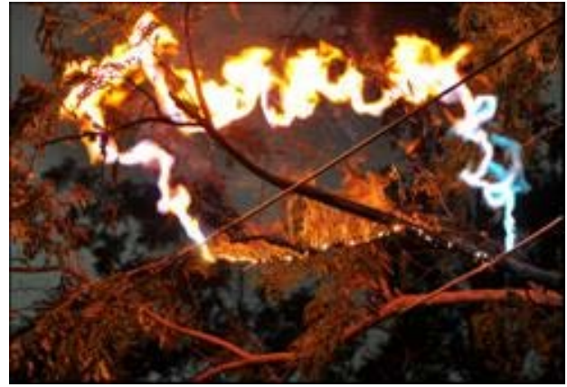
Photo 2: High voltage distribution phase/phase fault
