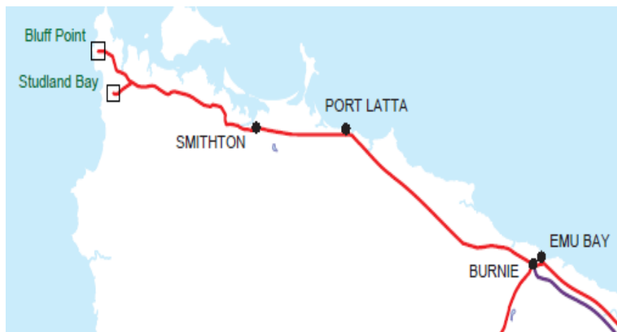
Figure 3: 110 kV transmission network from Smithton to the Bluff point and Studland Bay wind farms
