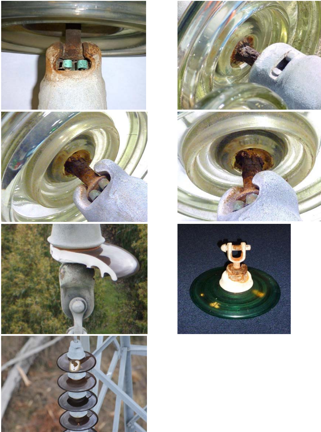
Figure 9: Typical defective insulators
