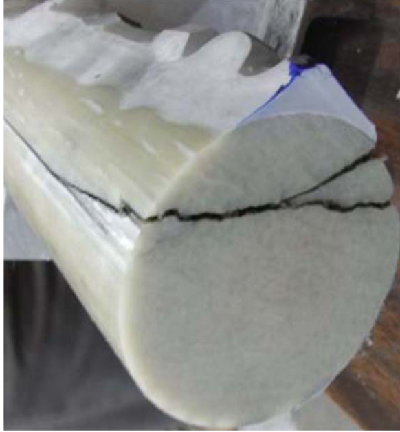
Figure 10: Cracking of fibreglass rod of insulator on TL446T232 (2013 failure) 3
