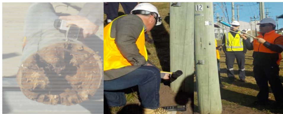
Figure 12 Non-Destructive Testing Methods for minimising need for wood drilling
