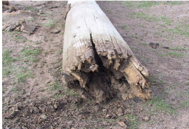
Figure 25: a wood pole that has failed in service
