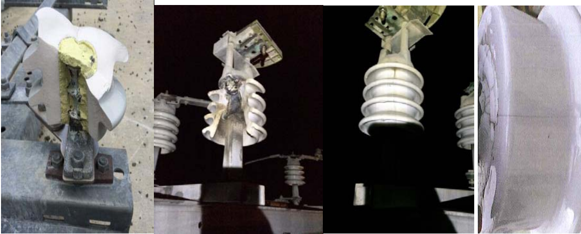
Figure 13: Air break switch porcelain insulator pin failure examples found in service
