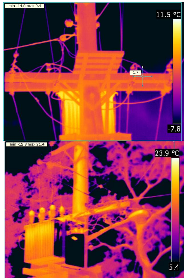
Figure 13: Thermal images showing warm transformer radiators and no hot spot defects
