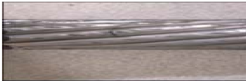
Figure 22 shows example of fretting conductor fatigue failure risk in AA or ACSR conductor
