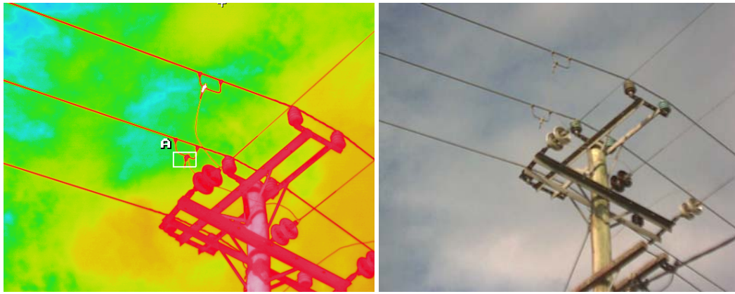
Figure 27: A Live Line Clamp through a thermal imaging camera and a normal camera
