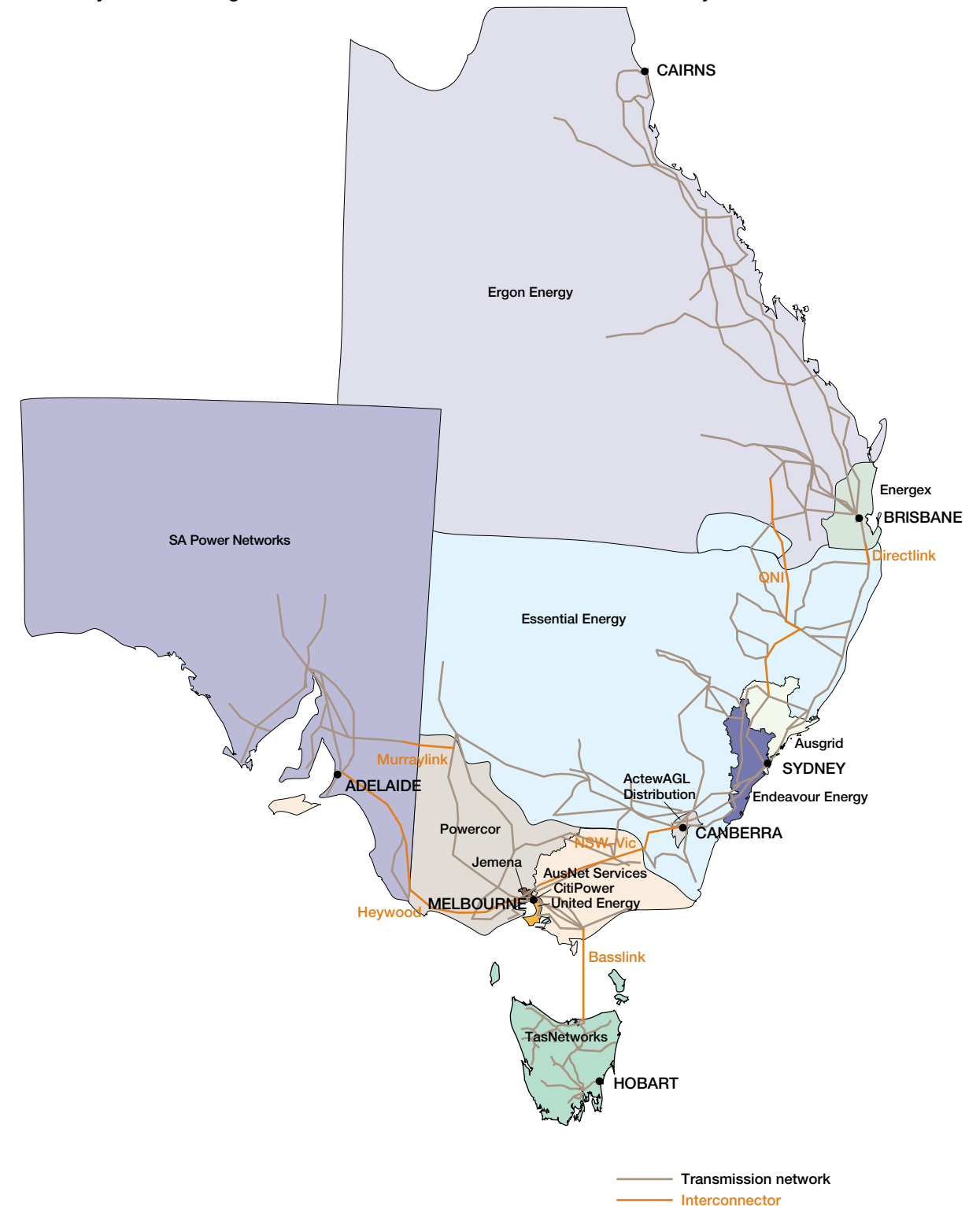
Figure 2.1 Electricity transmission grid and distribution networks in the National Electricity Market
