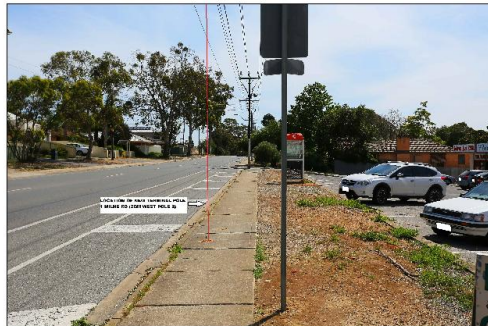
POLE 1 PROPOSED LOCATION OF POLE IN MILNE ROAD. PROPOSED 11,000-VOLT, LOW VOLTAGE & FIBRE OPTIC CABLES TO POLE 8.
