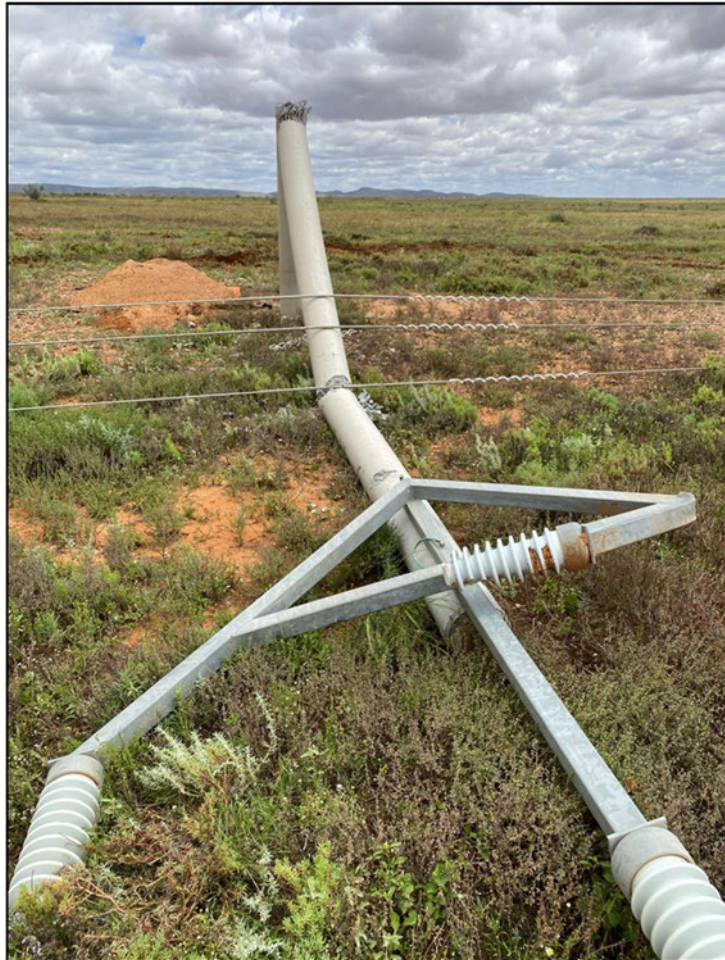
Figure 3 - Concrete Pole Failures INCD-38007-x
