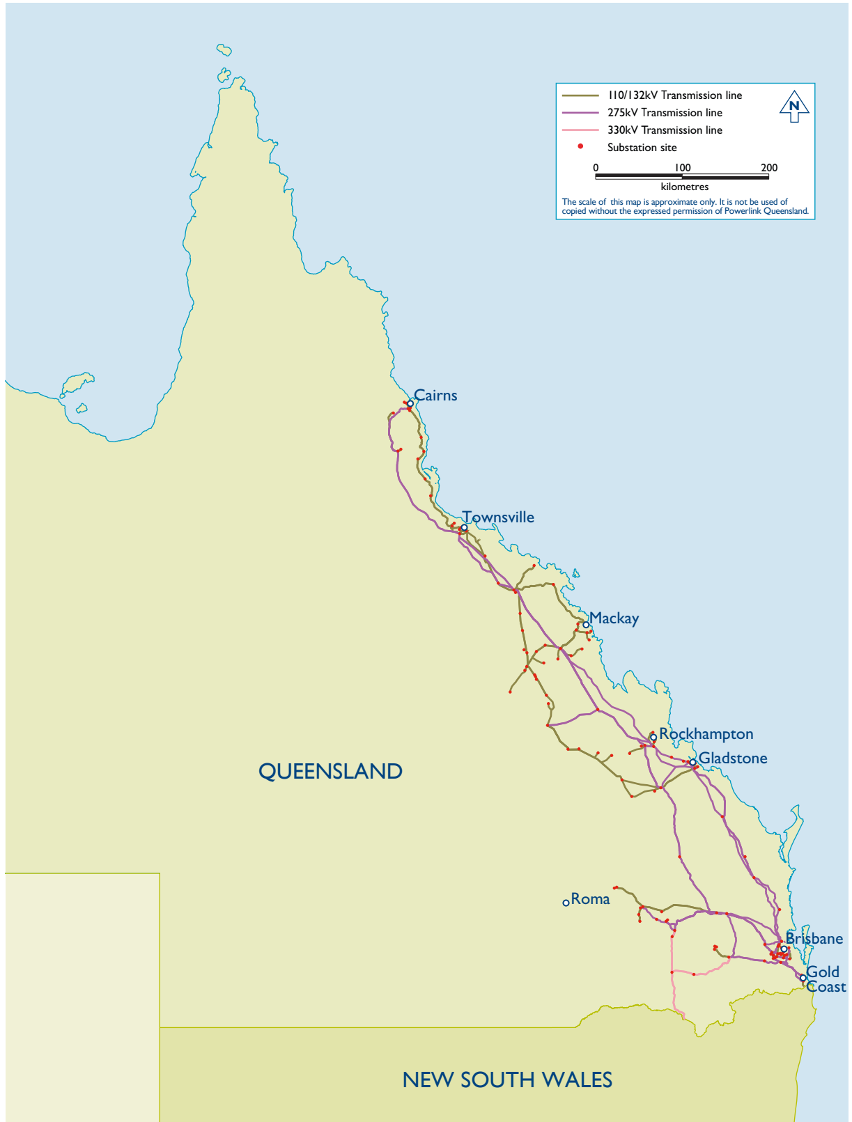
Figure 3.1 Existing Powerlink Queensland transmission network June 2015
