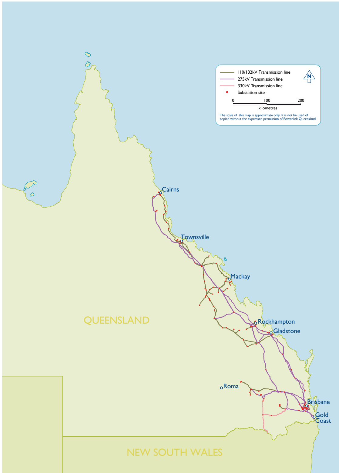
Figure 9.1 Existing Powerlink Queensland transmission network October 2020
