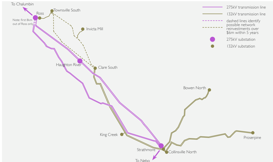
Figure 5.5 Southern Ross zone transmission network
