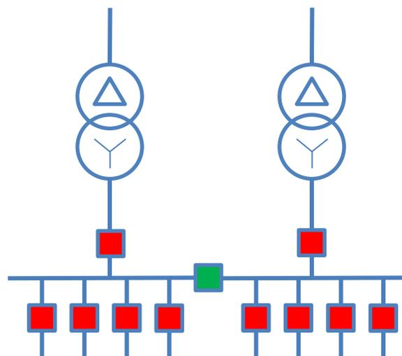
Figure 7 - Open 22kV Bus Tie Arrangement
