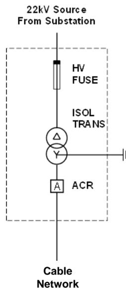
Figure 9 - Isolation Transformer Concept
