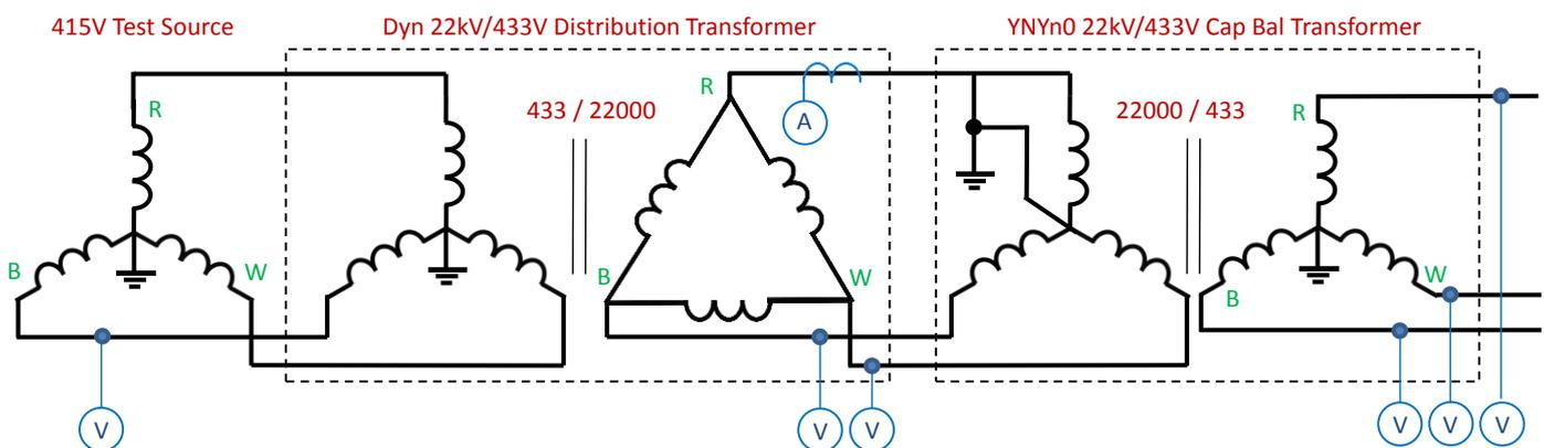
Figure 11 - Excitation Test Arrangement of Three Phase 22kV/433V Capacitive Balancing Transformer
