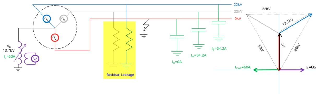
Figure 3 - Earth Fault in a Resonant System
