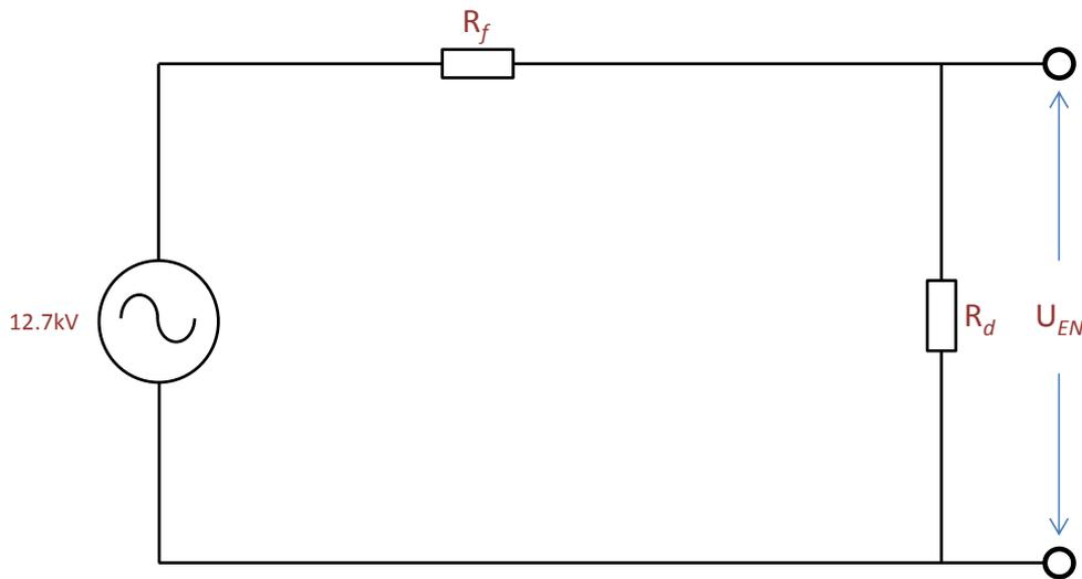
Figure 6 - Simplified Equivalent Circuit ( $Z_u = 0$ )
