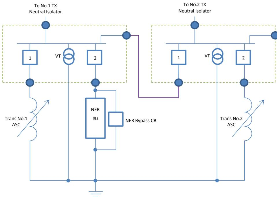
Figure 8 - Dual REFCL Neutral System Arrangement
