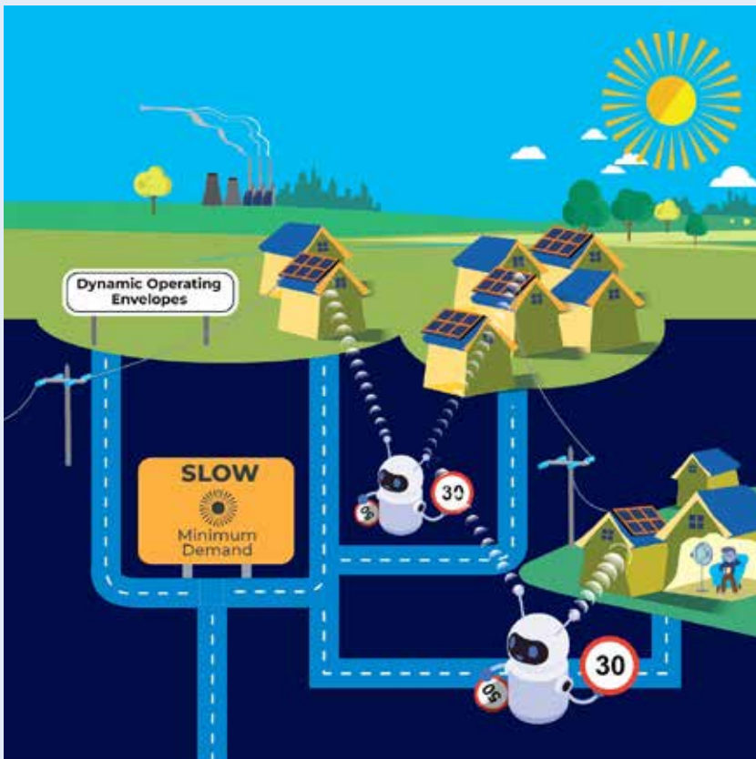
Figure 14 – Dynamic Operating Envelopes ramping down solar production on minimum demand days
