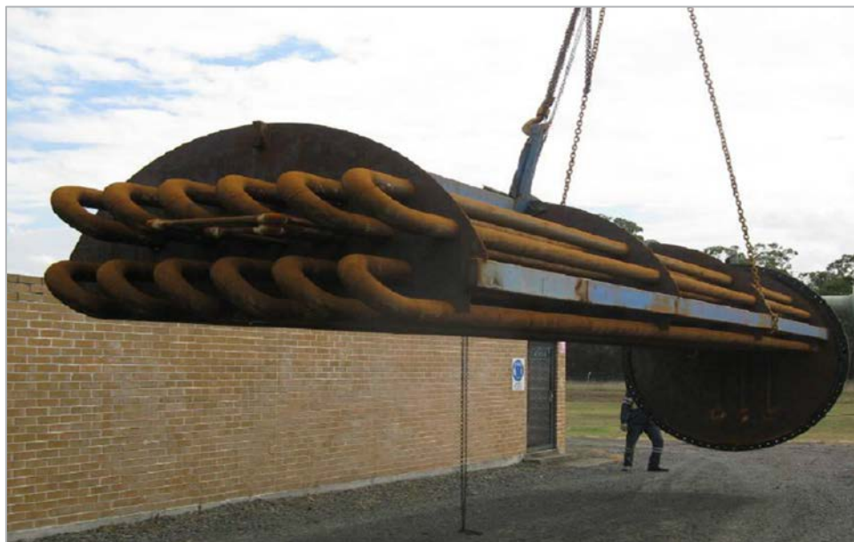
Figure 2-4: Fire tubes of a Water Bath Heater
