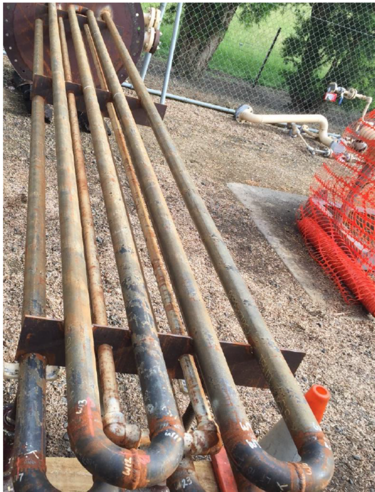
Figure 3-3: Process coils of the [REDACTED] Water Bath Heater
