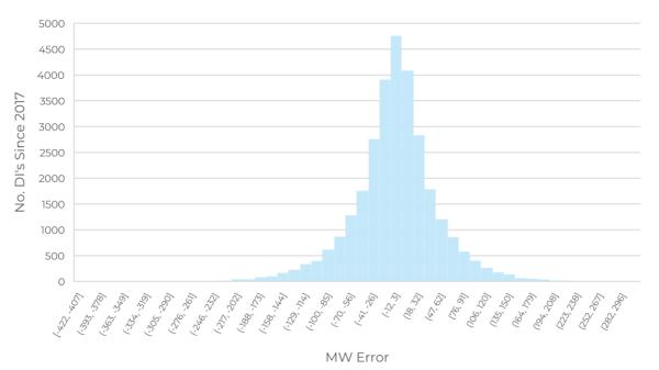
Curtailing the "overs" would result in a net-negative deviation, as shown in Figure 9 and Figure 10, requiring constant response from an ancillary service – either Regulation or Primary Frequency Control. Critically, curtailment would require greater Raise quantities of these services, with 10% of dispatch intervals since August 2019 having a -177 MW deviation from the forecast. A rule change that *causes* additional net-deviations may not be efficient,
