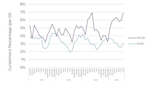
The AEMC recently made a temporary rule requiring a mandatory primary frequency response from all capable participants. Therefore, a curtailed wind farm would typically relax that curtailment when frequency was low (i.e., there was a shortfall of generation). Actual curtailment would therefore be roughly half this level.
