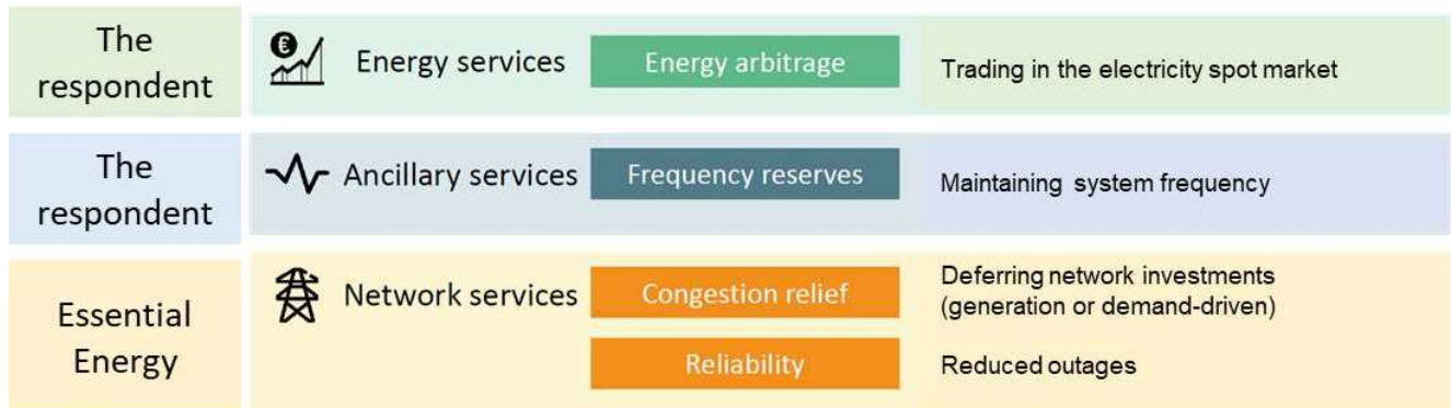
Figure 2: The value stack of market and network services provided by the battery
