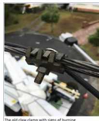
The old clamp with signs of burning
