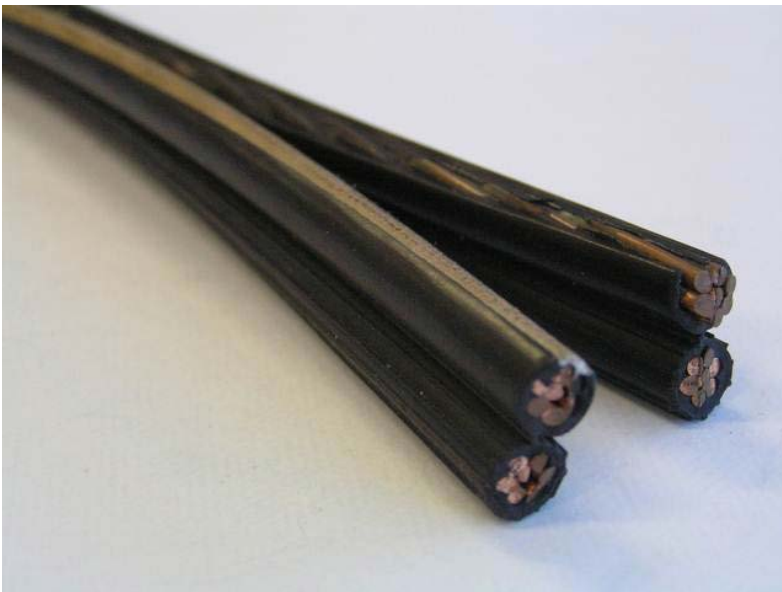
Figure 7: Deteriorated Colour Coded Service wire
