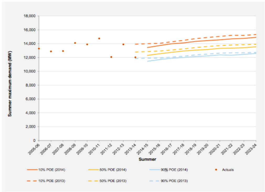
Figure 2: Summer 90%, 50% and 10% POE MD forecasts for NSW (source AEMO National Electricity Forecasting Report – June 2014)
