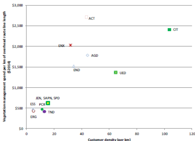
Figure A.18 Average vegetation management costs per kilometre of overhead line length for 2009 to 2013 against customer density ($2014)
