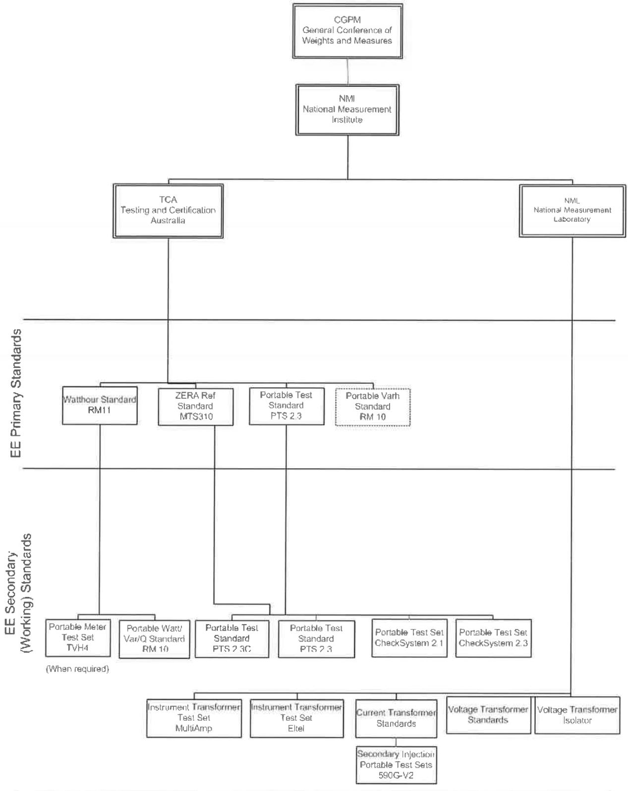
**Note:** PTS testing equipment are issued to Meter Technicians for field use.
