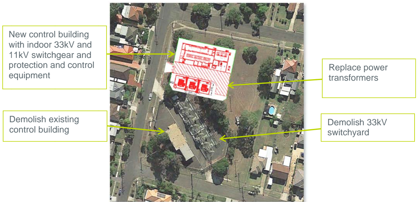
FIGURE 5 – NEW INDOOR SUBSTATION
