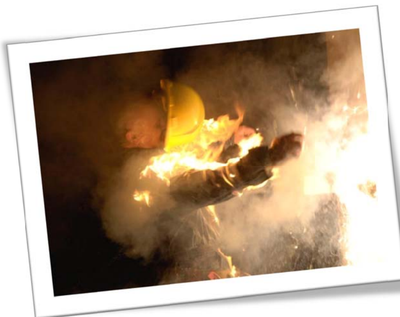
Aftermath of an arc flash explosion [2]
