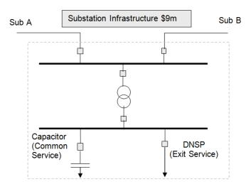
Step 1: The branches are Sub A, Sub B, DNSP, Tie Transformer and *prescribed common transmission services*.
