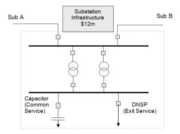
Step 1: The branches are Sub A, Sub B, DNSP, Tie Transformer 1, Tie Transformer 2 and prescribed common transmission service.
