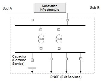
Step 1: The branches are Sub A, Sub B, *DNSP*1, *DNSP*2, *DNSP*3, Tie Transformer 1, Tie Transformer 2 and PCS.
