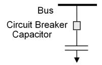
Branch with Capacitor, Circuit Breaker and Bus
