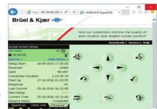
Fig. 7 View the results and status of the NMT remotely from a web browser
