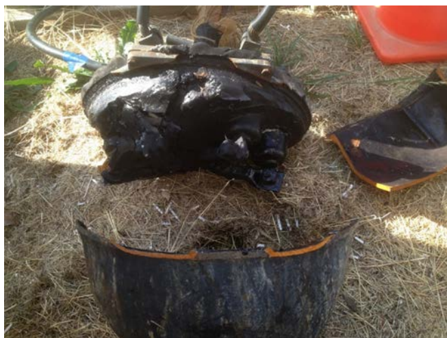
Figure 4 and Figure 5 Damage caused by explosive failure of cast iron LV pothead:
