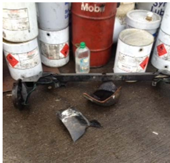
Figure 4 and Figure 5 Damage caused by explosive failure of cast iron LV pothead:
