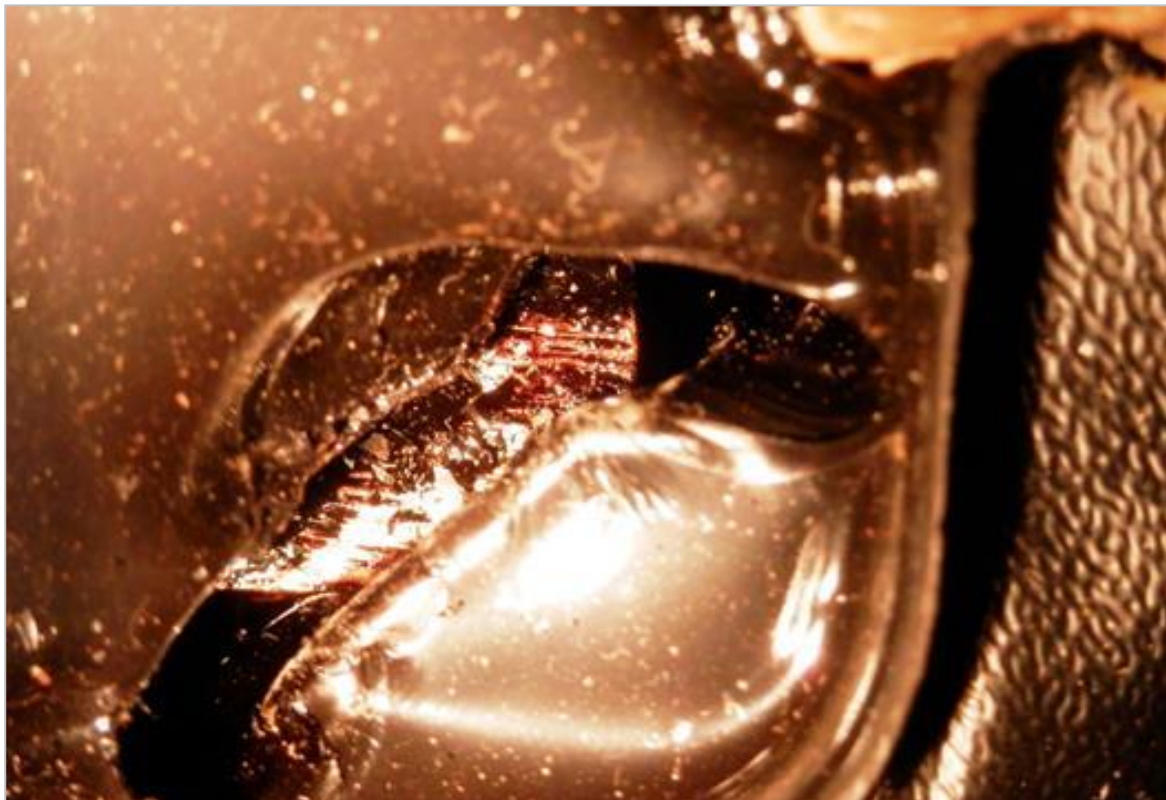
Figure 13 Example: void in compound insulation in bare busbar highlighting failed integrity of electrical insulation (2015)
