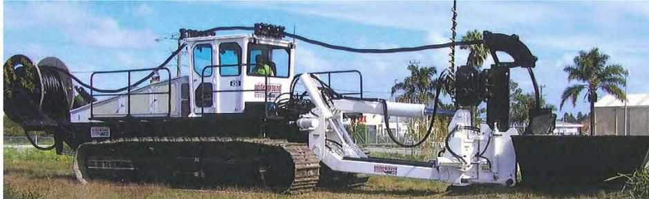
**Figure 20: Plough for undergrounding cable**
