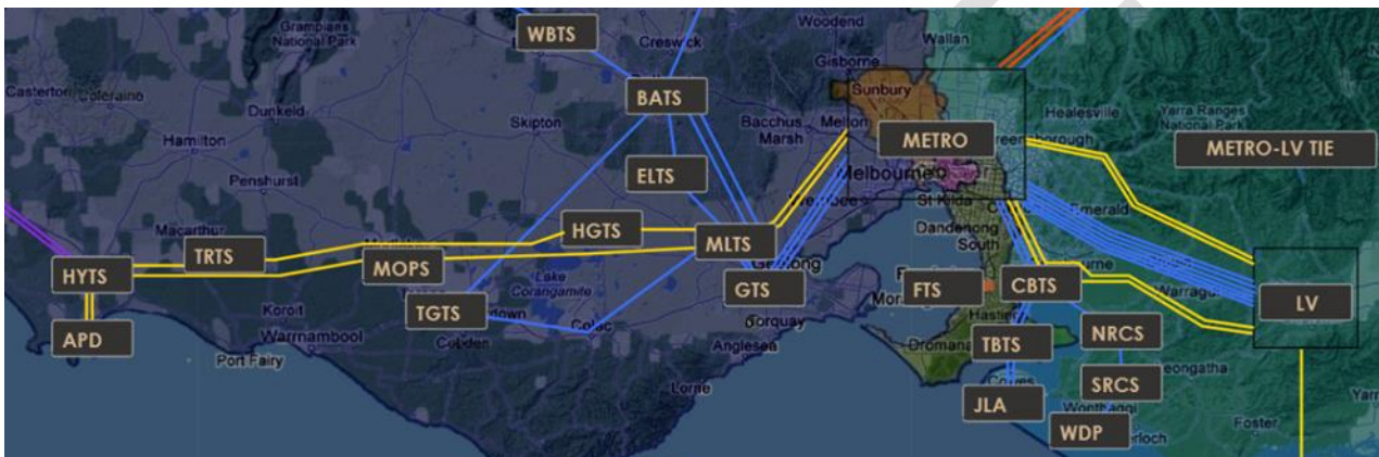
Figure 2 - 500 kV Transmission Backbone
