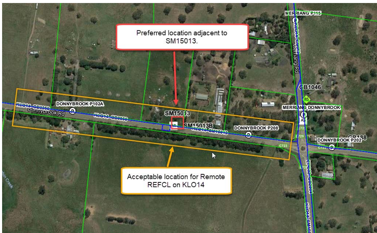
Fig 1. Proposed location for Remote REFCL on KLO14.
