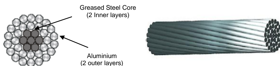
Figure 1. Typical ACSR Conductor
