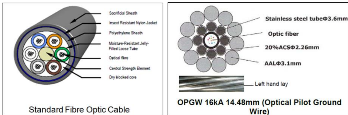
Figure 4: Typical cross-section of Fibre cable
