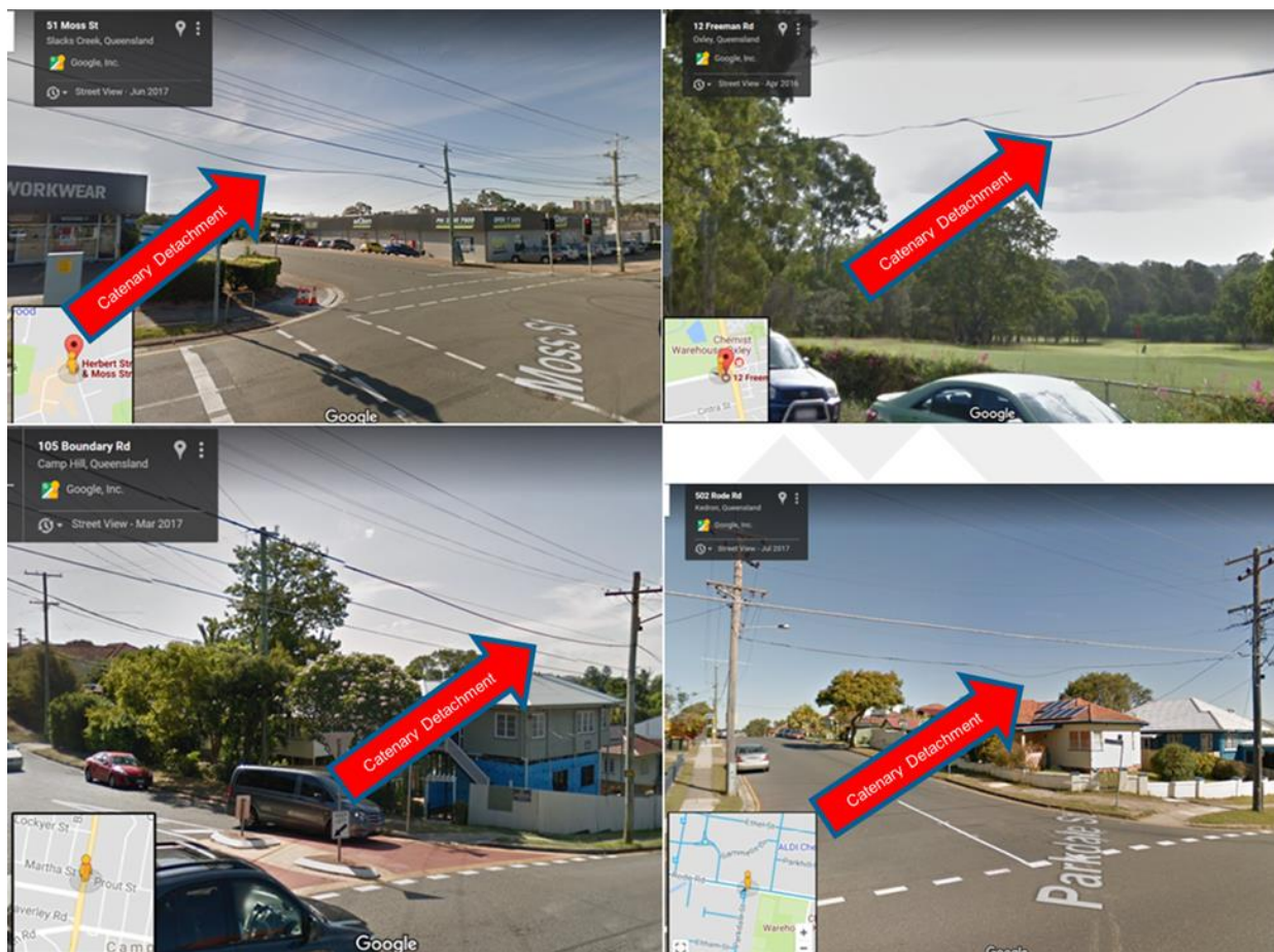
Figure 14: Catenary Detachments of Metallic Pilot cables
