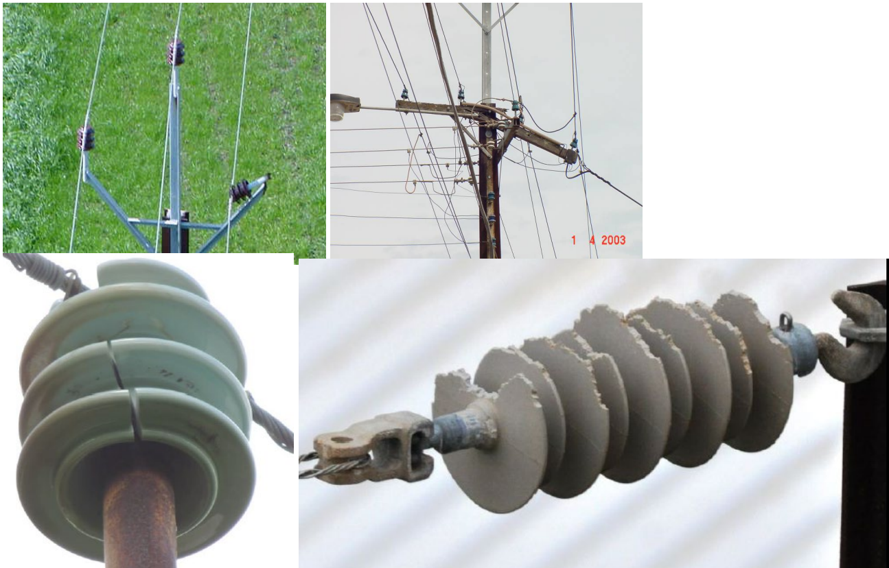
Figure 43 Typical defects of crossarms and insulators
