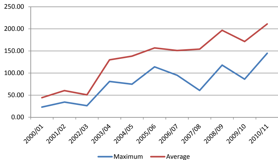
Figure 5 Temperature sensitivity coefficients, maximum temperature versus average temperature for South East Queensland (MW per °C)
