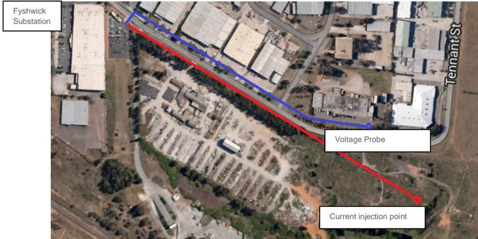
Figure 17 – Remote Earth or Test Current Electrodes
