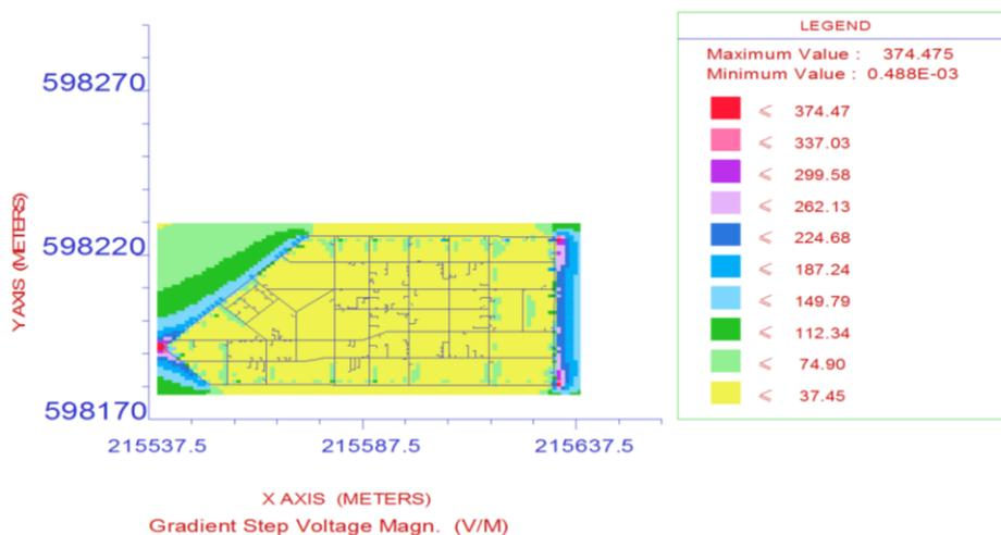
The safety limit for Step Voltages internal to the substation with public access for a 70kg body weight on yard stone is 2838V. The model indicates that these are within the permissible safe voltage limit.
