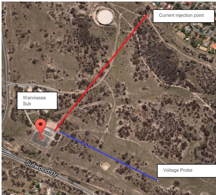
Figure 18 – Remote Earth or Test Current Electrodes
