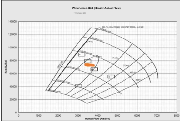
Operating points in optimal location in wheel map.
