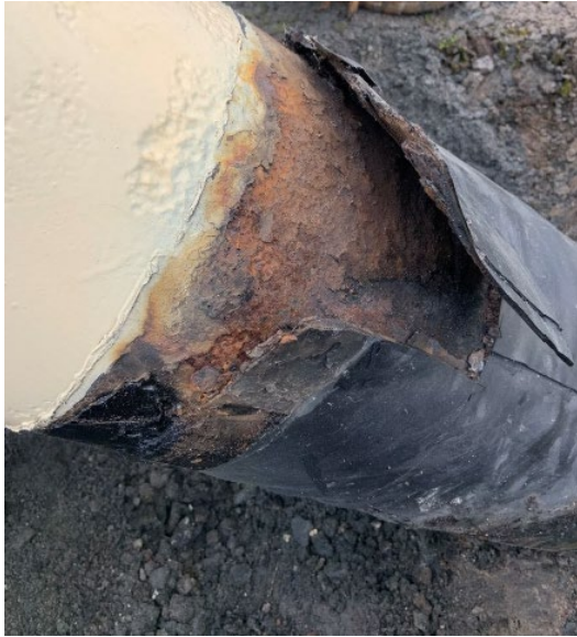
Left: Typical MLV site valve bypass piping corroded.
