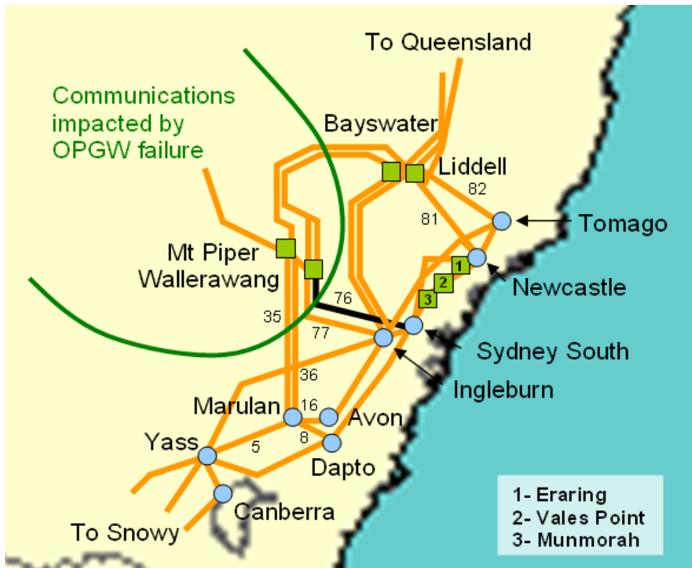
Figure 1: Line 76 and the area affected by the communications failure
