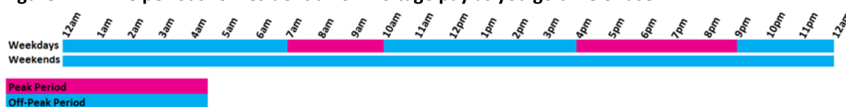
Figure 1: Time periods for residential low voltage pay as you go time of use
